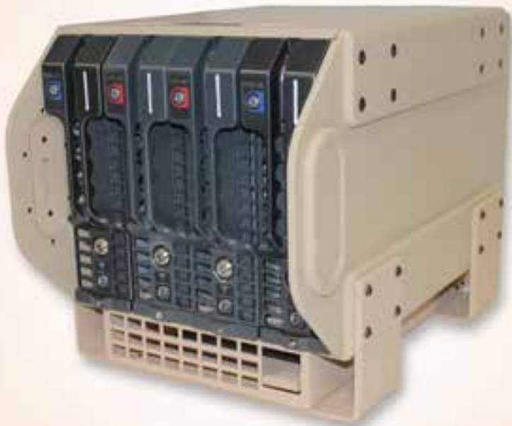
EQUINOX Next Generation is the latest vehicle based Electronic Countermeasure (ECM) system from Allen-Vanguard
